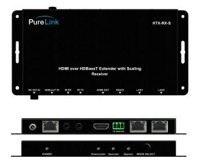
Designed as a simplified extension solution for the HTX Series matrix switchers, the HTX-RX-S provides highperformance up/downscaling capabilities at Ultra HD/4K resolutions, extending uncompressed HDMI video, audio, full 3D content, as well as bi-directional control to distances up to 330ft. (100m).
